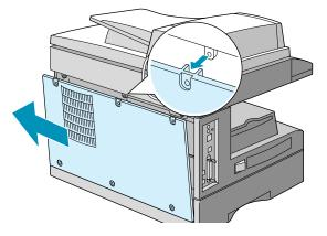
**5** Remove the one screw from the port cover.
